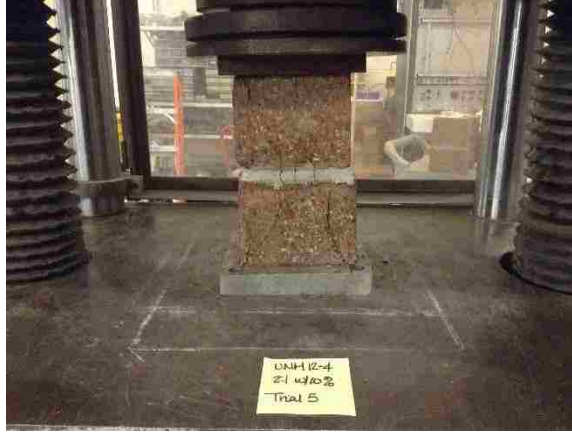
Figure 3. 34. SCEB 7 prism compression on Tinius Olsen machine.
