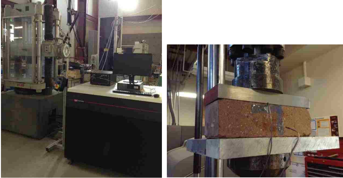
Figure 3. 22. (a) 400 kip capacity Tinius Olsen machine, Model No. 139000 (b) SCEB dry compression test to determine Poisson's Ratio on 120 kip capacity Instron machine, Model No.AW2568-3.
