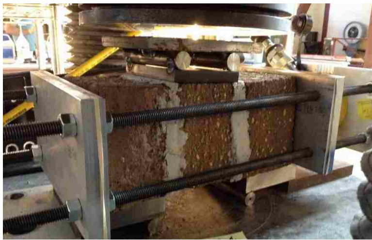
Figure 3. 42. SAB prism in shear testing apparatus in the Tinius Olsen machine.
