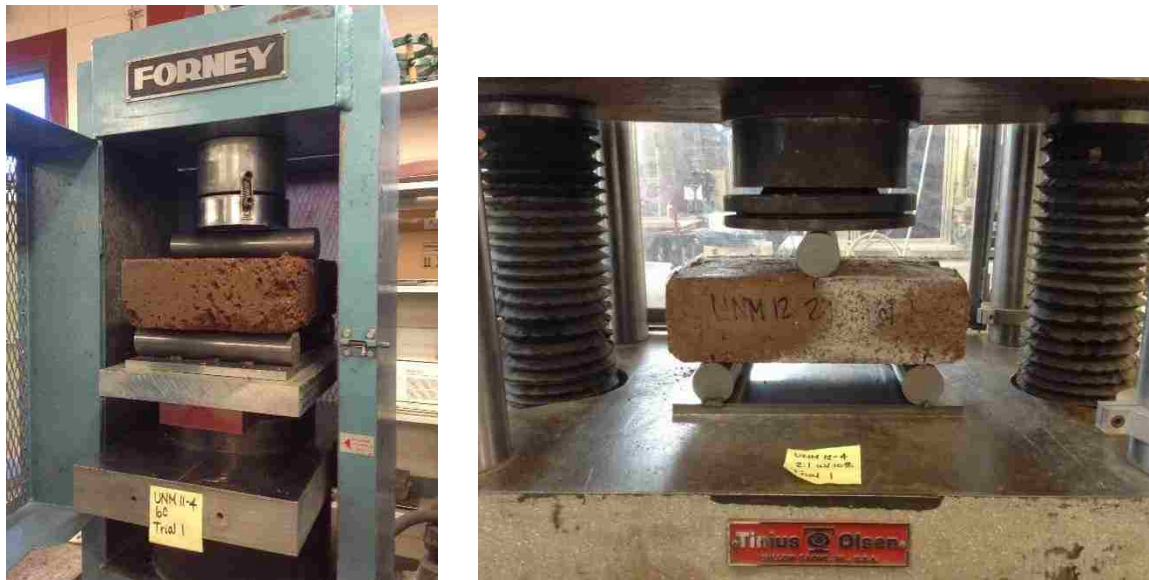
Figure 3. 24. (a) Saturated SCEB 4 tested for MOR on Forney. (b) Saturated SCEB 7 tested for MOR on Tinius Olsen.
