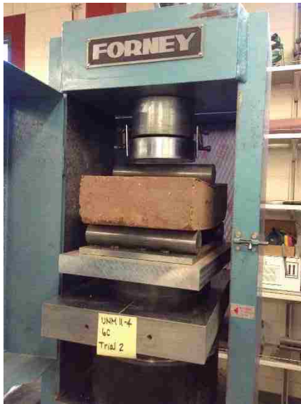
Figure 3. 23. (a) SCEB 4 tested for dry MOR on Forney. (b) SCEB 7 tested for dry MOR on Tinius Olsen.
