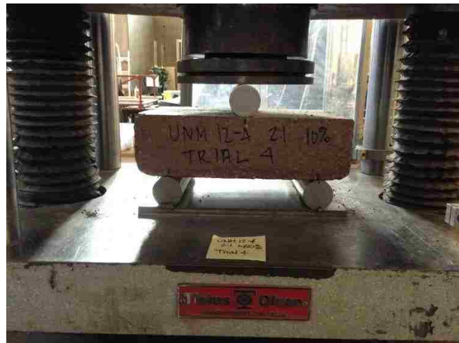
Figure 3. 23. (a) SCEB 4 tested for dry MOR on Forney. (b) SCEB 7 tested for dry MOR on Tinius Olsen.
